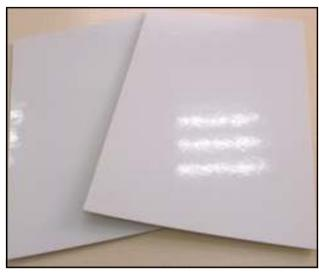
Carbon-Core Composite Panels comes with a 8mm cell size core. The honeycomb core has an 18oz layer of resin mixed with fiberglass on each side and all of the panels have a white glossy look to them, although sanded panels are available.
